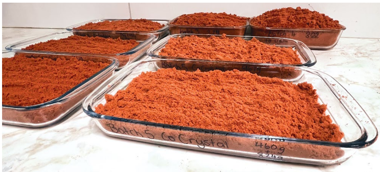
Figure 3 – Cobalt sulphate produced at the Broken Hill Technology Development Centre Plant
