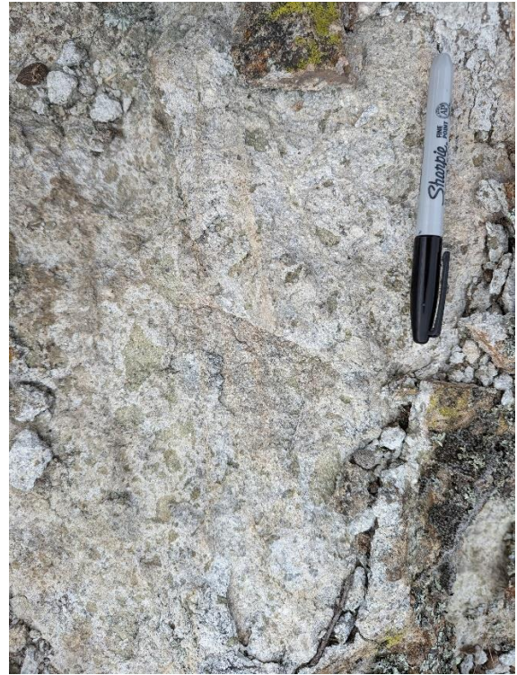
Figure 7: strongly clay altered pyroclastic volcanic (sample 72432).
