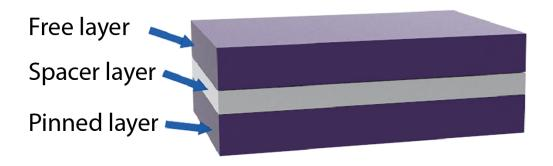
**Image 1:** Example magnetic tunnelling junction. Quantum tunnelling allows electrons to move between two ferromagnetic layers (free and pinned layers) separated by an insulating barrier (spacer layer). The sensor detects resistance changes, corresponding to changes in the magnetic field. The ability of electrons to quantum tunnel between layers based on their magnetic alignment gives the TMR sensor its high sensitivity and efficiency.
