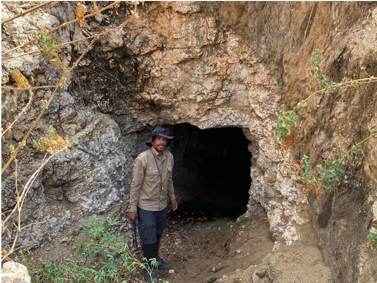
Figure 4. Artisanal mine for beryl in an estimated 5-metre-wide NNE trending pegmatite in the NE tenement in the Bandarra-São Braz tenements
