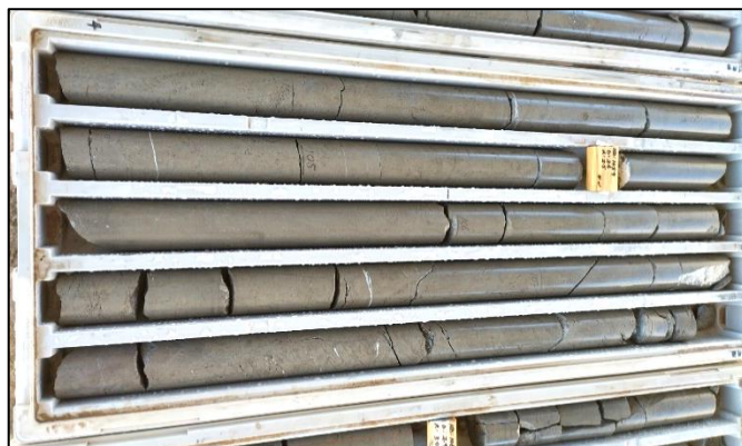
Hole PGNL005 103.7 – 107.9m: 4.2m interval of Massive Sulphide Pyrite dominant core assaying 4.2% lead, 9.10% zinc, 449g/t silver, 0.97g/t gold and 0.09% copper.
