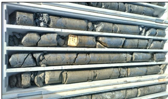
Hole PGNL003 113.1 – 116.5m: 3.4m interval of Massive Sulphide Pyrite dominant core assaying 17.2% lead, 7.4% zinc, 463g/t silver, 0.94g/t gold and 0.1% copper.
