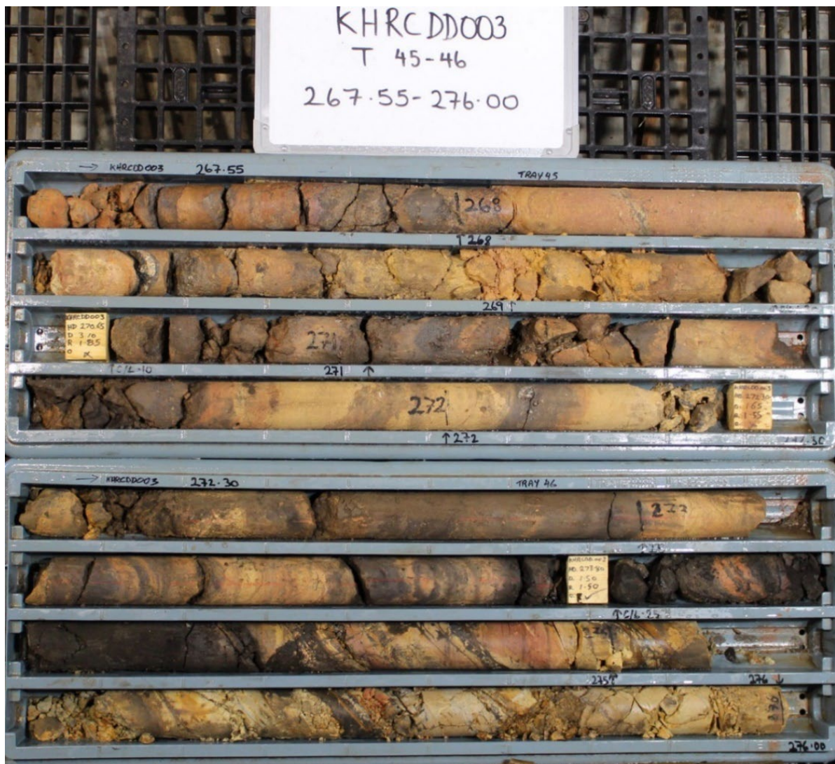
Figure 4: Ferruginous-gossanous oxidised Preston Formation sediments, KHRCD003. Refer to Table 1 for assay grades.
