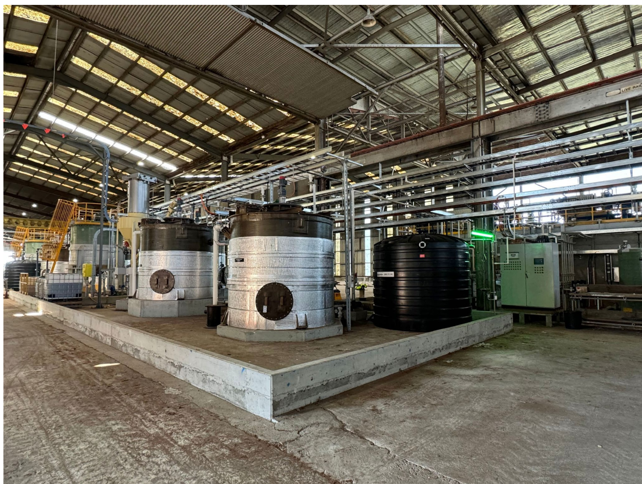
Figure: Hydromet piping modifications and installation new surplus capacity tanks completed
