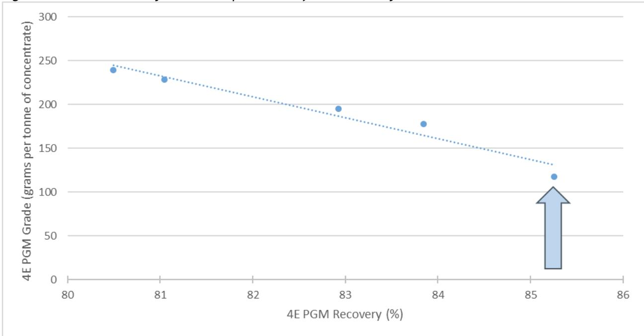
Subsequent rougher kinetic testwork which was conducted with an optimised reagent suite, delivered a result of 85% recovery on a 6E basis. It is noted that this subsequent test did not test the cleaning of the rougher concentrate. The concentrate grade is not reported as it is not a locked cycle test. The financial model uses a 6E recovery of 85% and a 6E grade of 100 g/t.
