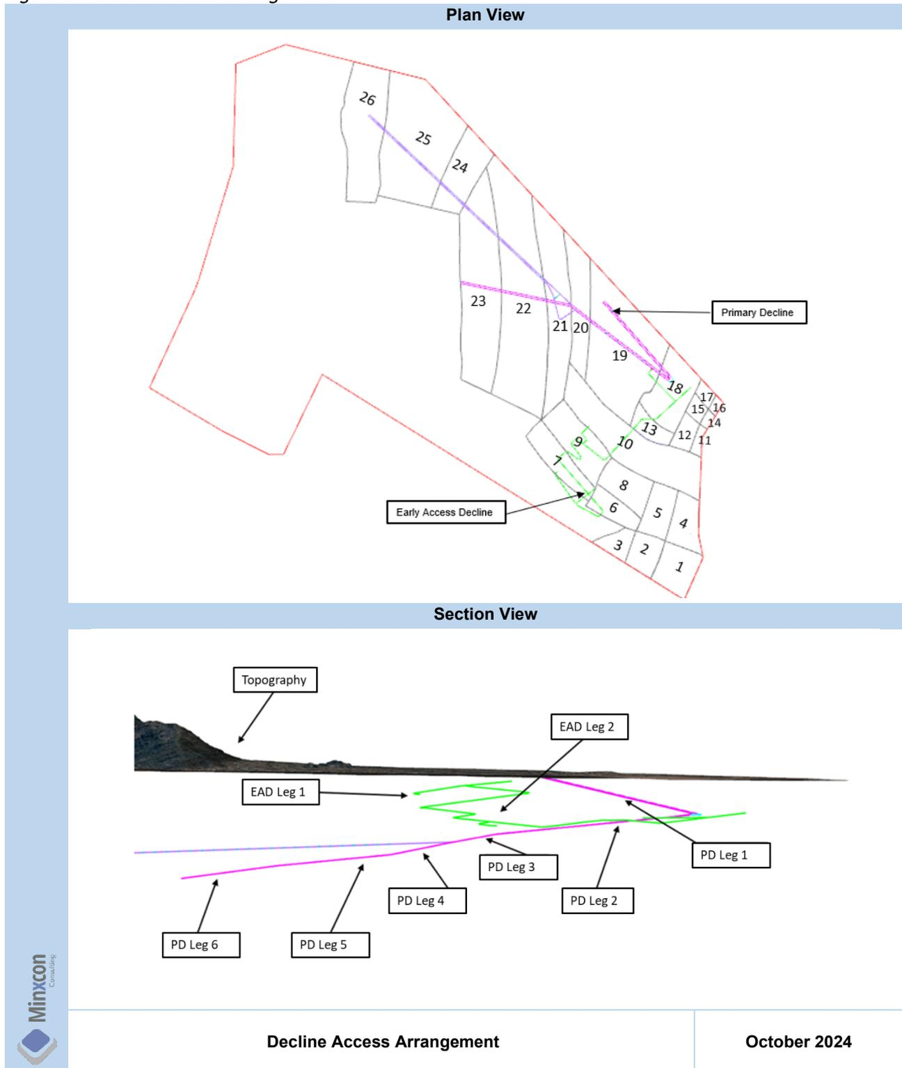
Due to the characteristics of the deposit, variations in dip inclination are observed throughout the orebody. Consequently, the decline is divided into distinct sections to accommodate these different dip angles. To ensure comprehensive access to the entire orebody, two independent declines, the PD and the EAD are required. These separate declines are interconnected at block 19, facilitating efficient movement between them and enhancing overall operational flexibility.
