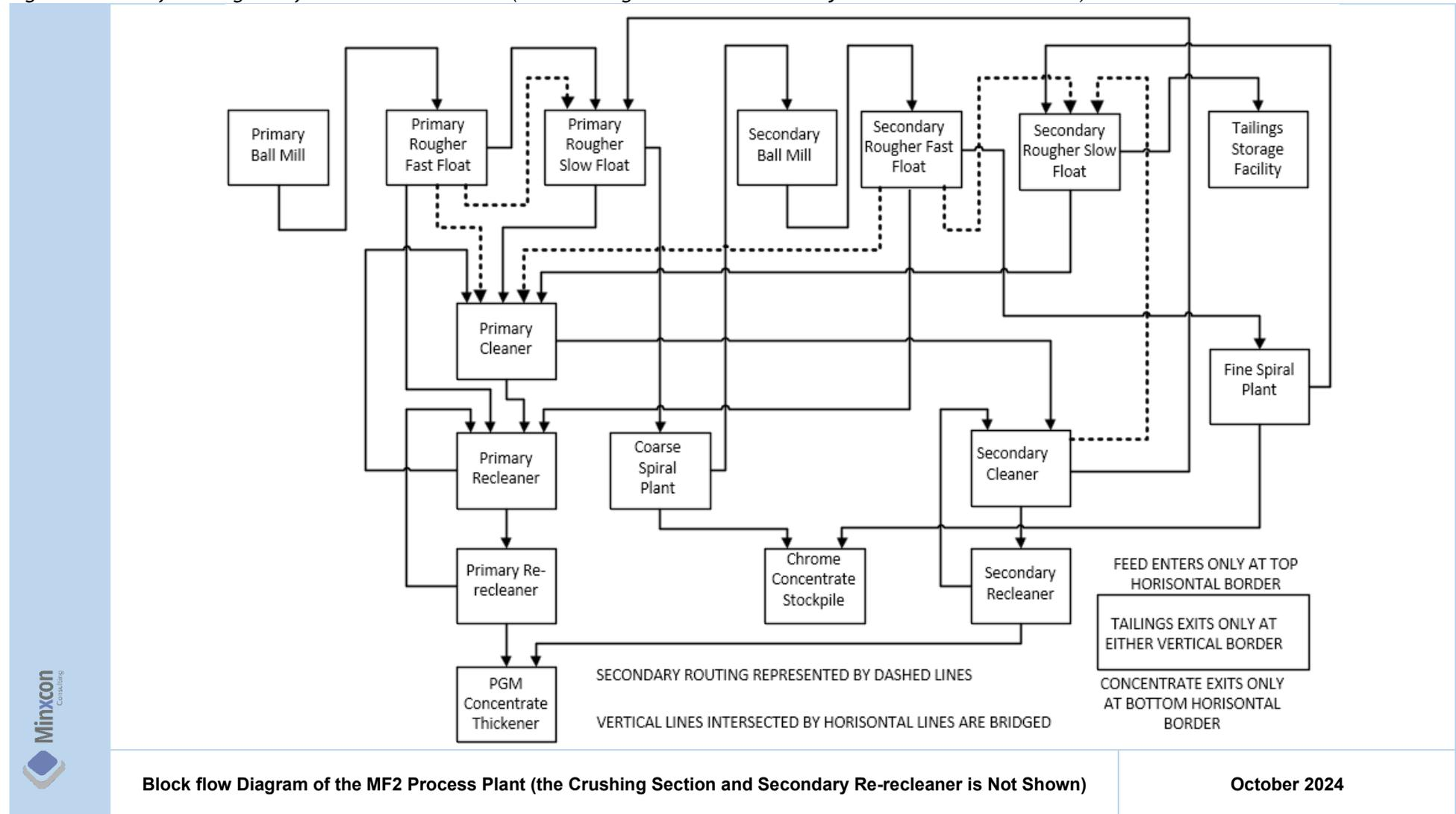
Figure 43: Current Bengwenyama Process Flow Diagram (Crushing & Secondary Cleaning Circuit Not Shown to Enhance Clarity)
