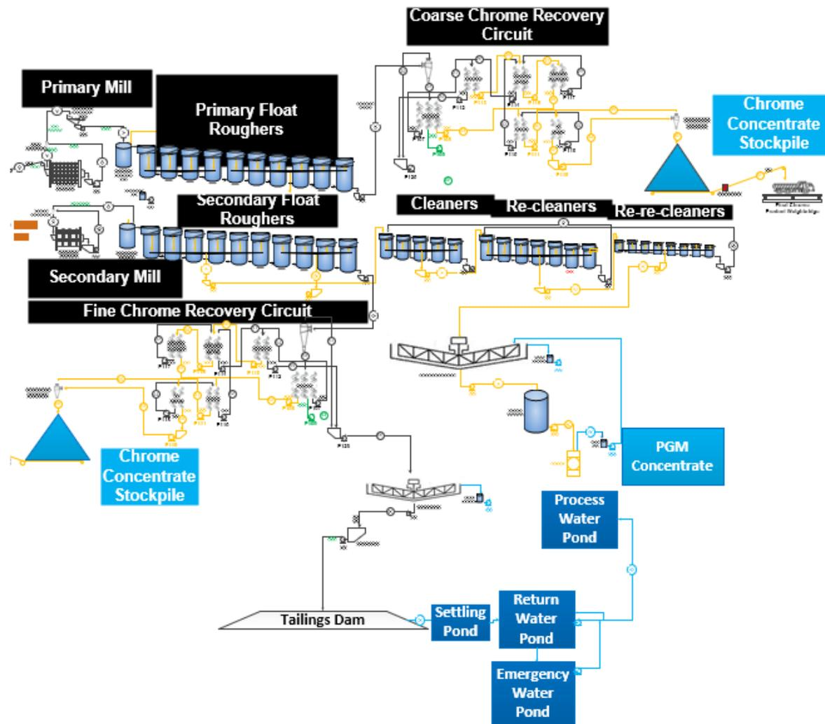
Current Bengwenyama Process Flow Diagram (Crushing & Secondary Cleaning Circuit Not Shown to Enhance Clarity)
