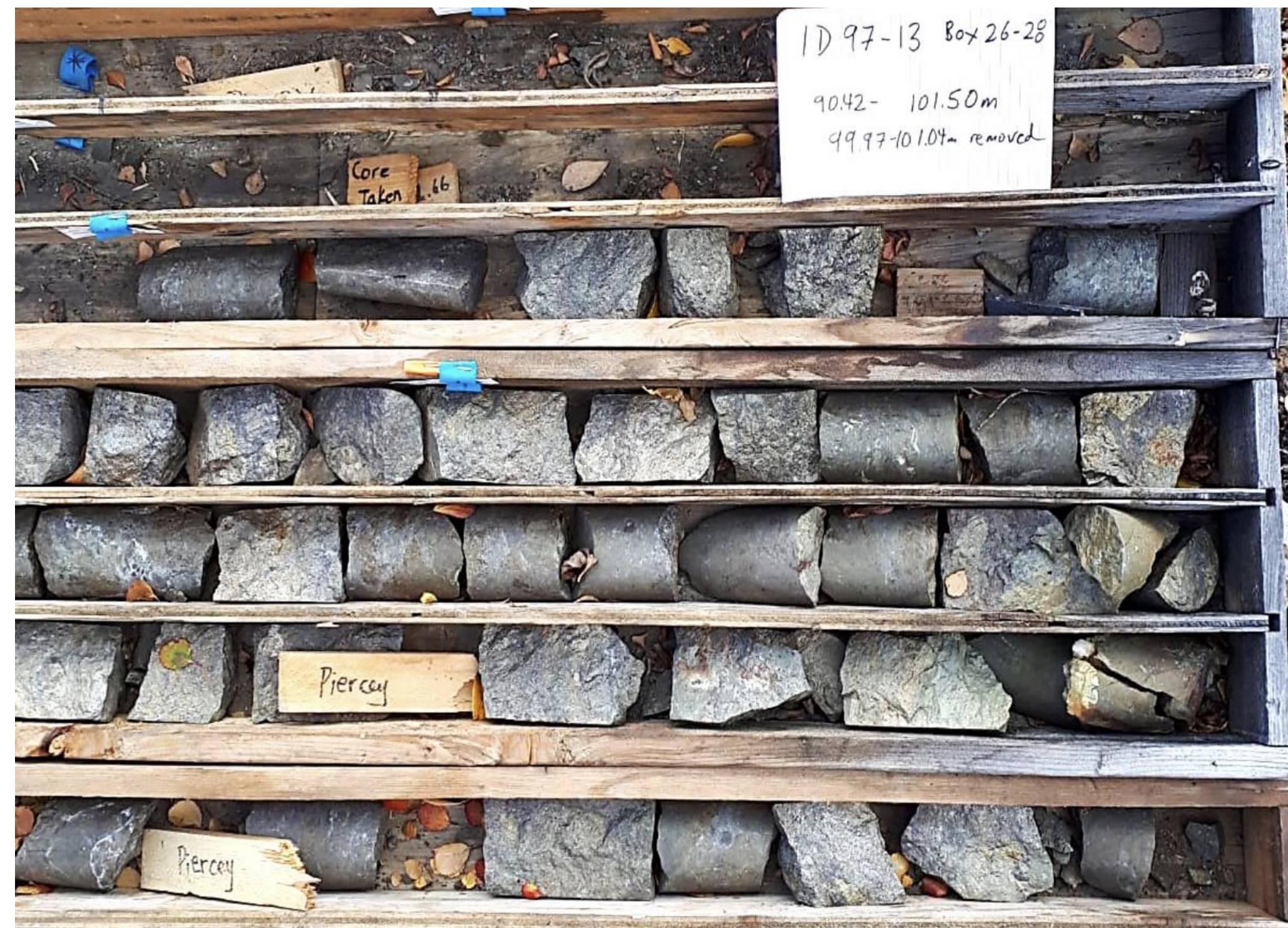
Figure 3: ID97-13 90.42-10 Core trays from the historical drilling prior to resampling. Semi-massive sulphide concordant with host unit bedding, with 3 to 10% chalcopyrite and up to 5% pyrite throughout the interval. Copper concentrations over the interval 90.42-101.5 m from 1.06 to 3.15% copper, 0.04 to 0.27 g/t gold (not all assayed for gold). 376943 East/ 6862786 North. UTM Zone 9 and original project NAD27 datum.
