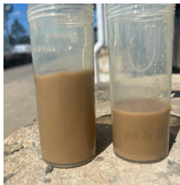
Figure 4: Cyclone overflow (left) and underflow (right) products from cyclone testing.
