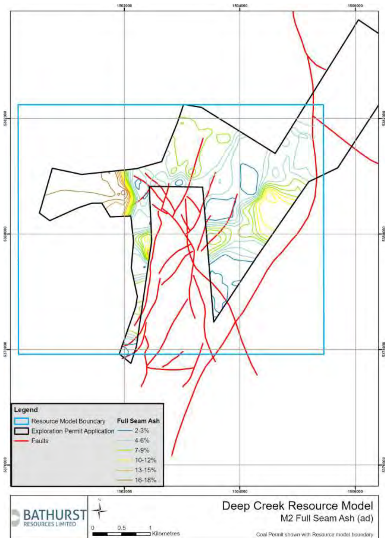
Figure 10: Plan showing in-situ full M2 seam ash on an air-dried basis across the Deep Creek resource area
