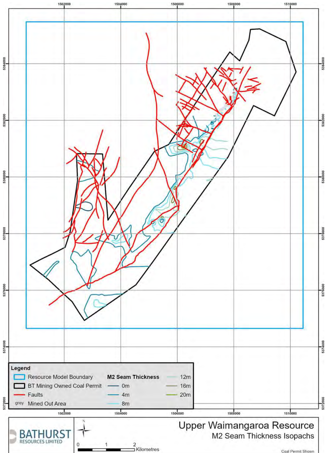
Figure 9: Plan showing full seam thickness (M2 Coal Seam) contours
