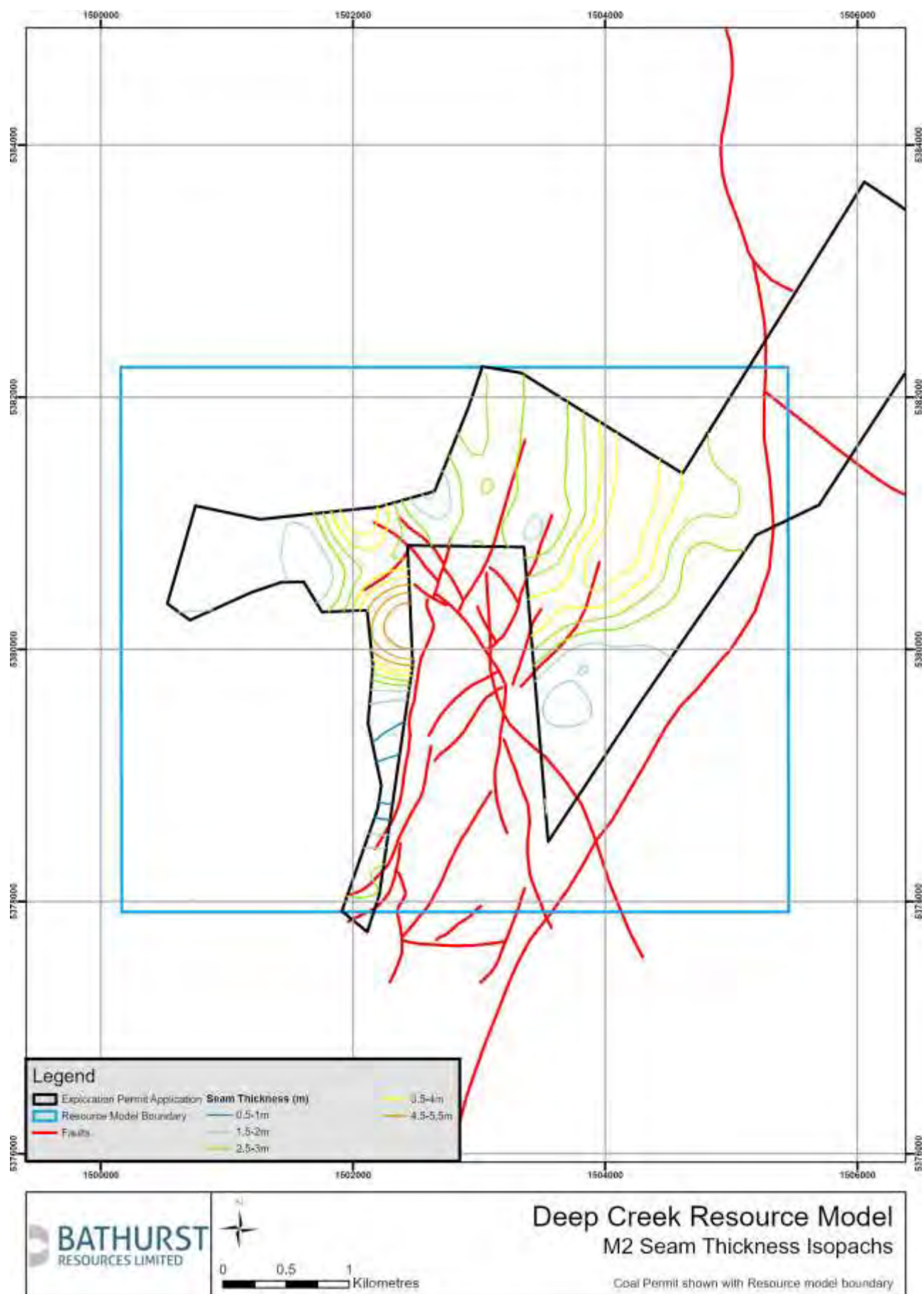
Figure 9: Plan showing full seam thickness (M2 Coal Seam) contours for the Deep Creek area
