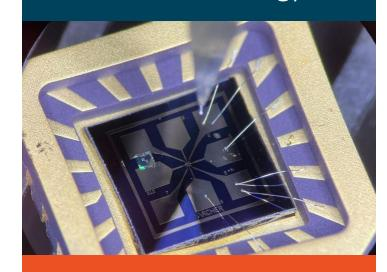
A carbon-based quantum device for applications like sensing and computing and the possibility of integrating with other electronics.
