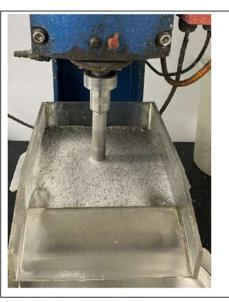
Fig 1. Photo FT\_H3 sample (Con1) at start of Test Vs 10 minutes of float time (Con4) Core Metallurgy Report
