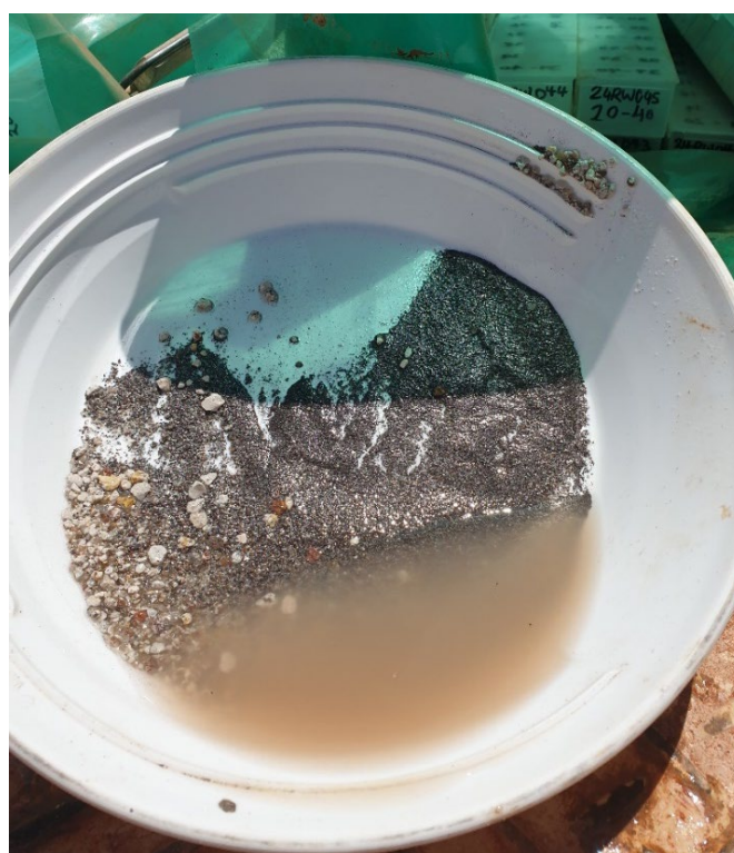
Photo 2 – Panned Heavy Minerals from drill hole 24RW049, (10-11 metres). HM estimate based solely on visual inspection is 20% and is yet to be assayed. No identification of the HM species can be made until laboratory work is completed. Results are expected in 4 to 6 weeks' time. Refer to Table 4 at the end of this report for further Cautionary Statement details.
