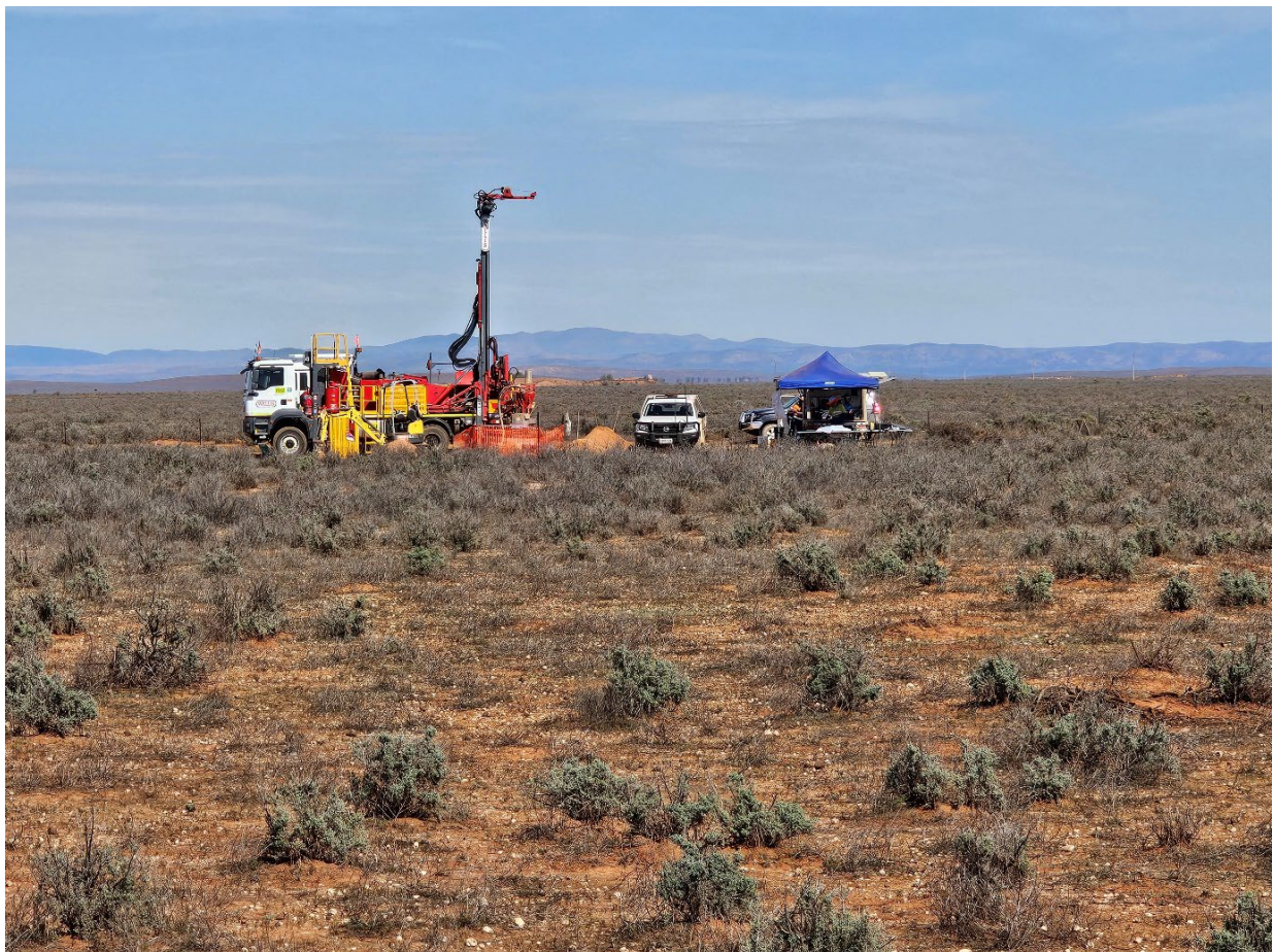
Figure 6: Air Core drilling at Target Area 1.
