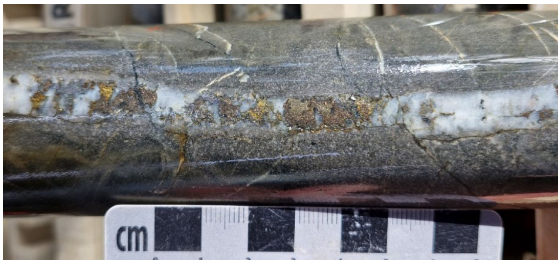
Figure 10: CUTAD01, 225.3m - Unmineralized pyrrhotite (brown-bronze)-chalcopyrite (yellow)-pyrite (brassy yellow) in quartz vein (see Appendix 1, Drill Log Summaries and Figure 3 Cautionary Note Page 2).
