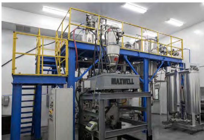
Cathode Pilot Line with nameplate capacity of 10 tpa
