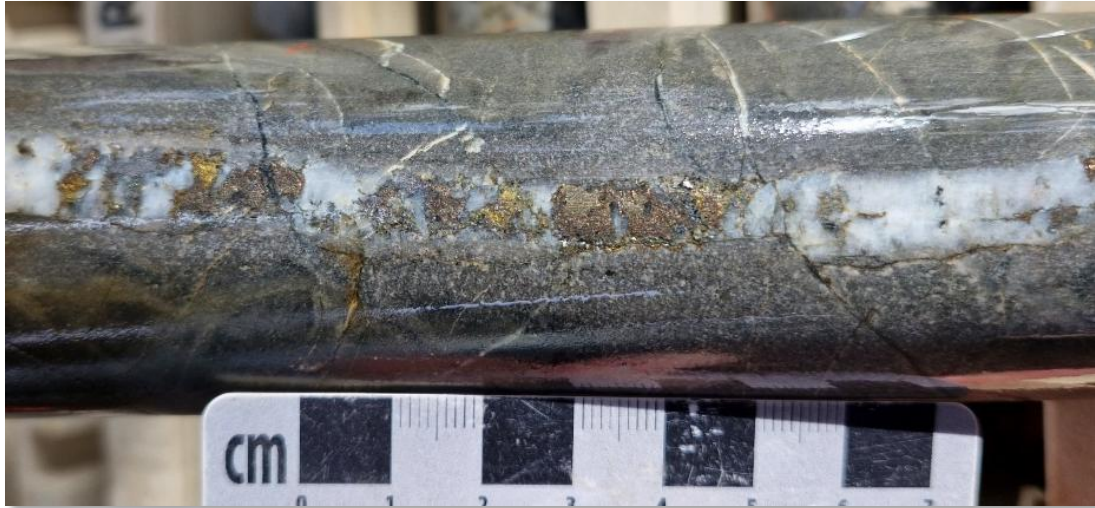
Figure 10: CUTAD01, 225.3m - Unsampled pyrrhotite (brown-bronze)-chalcopyrite (yellow)-pyrite (brass yellow) in quartz vein (see Appendix 1 & 2, Drill Log Summaries and Cautionary Note Page 2).
