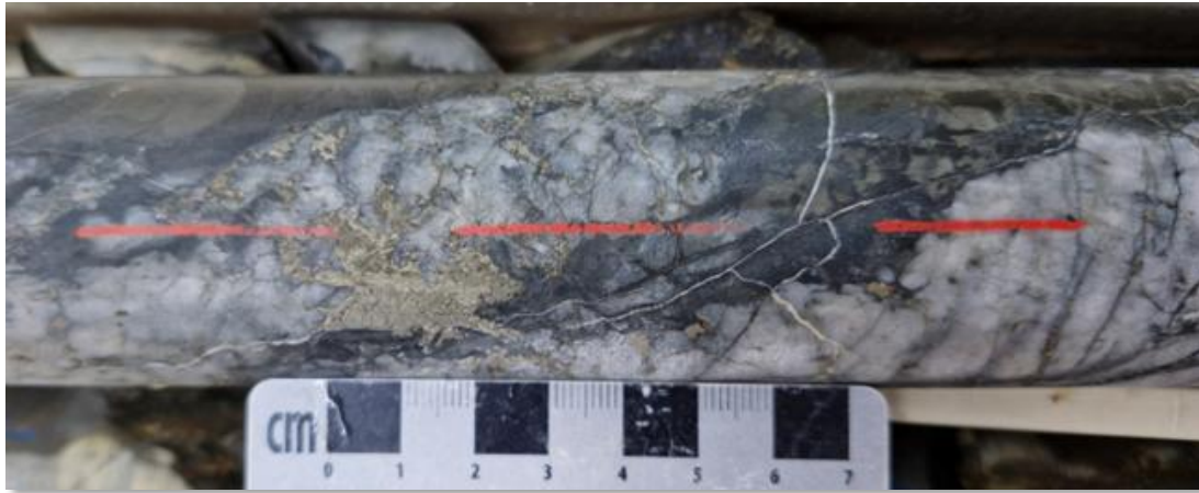
Figure 4: CUTBD03, 145m – Unsampld pyrite(brass-yellow)-pyrrhotite (brown-bronze) in quartz vein (see Appendix 1 & 2, Drill Log Summaries and Cautionary Note Page 2).
