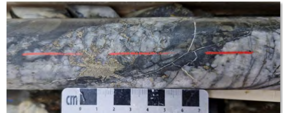
CUTBD02, 419.8m – Unsampled arsenopyrite (grey) in quartz vein 1
