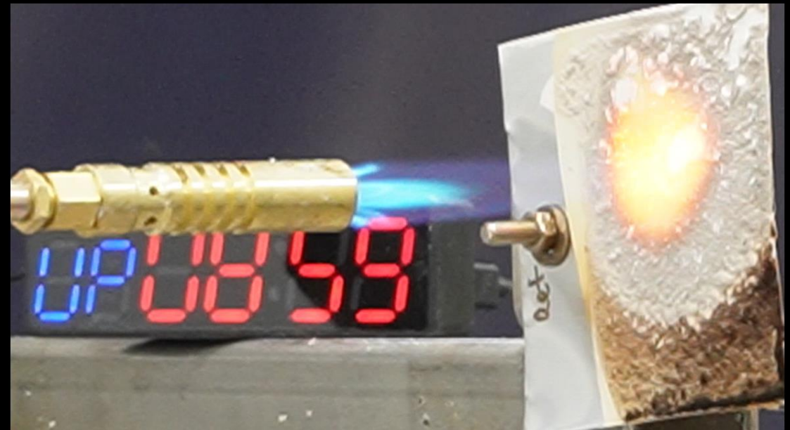
ULTRA-COATED ALUMINIUM Layer integrity intact after 9 minutes under butane flame
