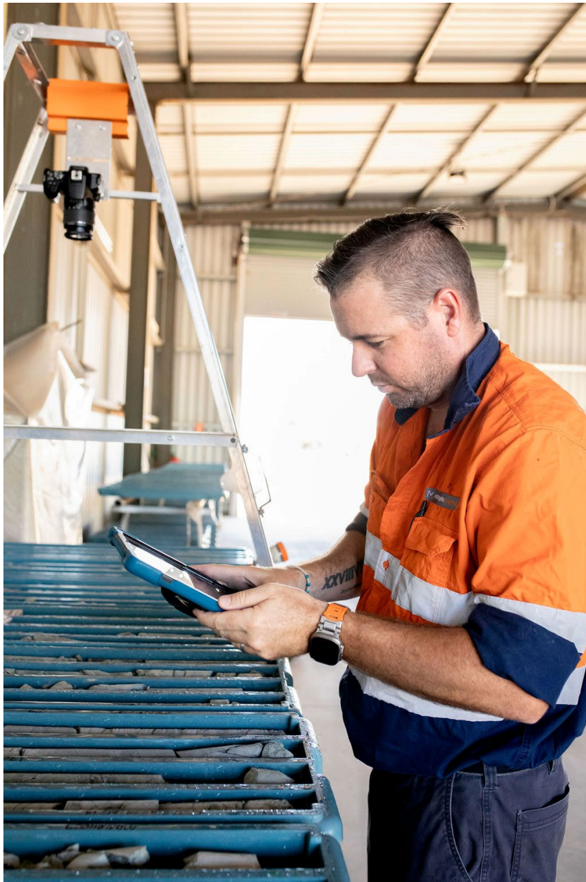
Figure7. Field Technician Matt Ellis photographing drill core as part of the core assessment process.
