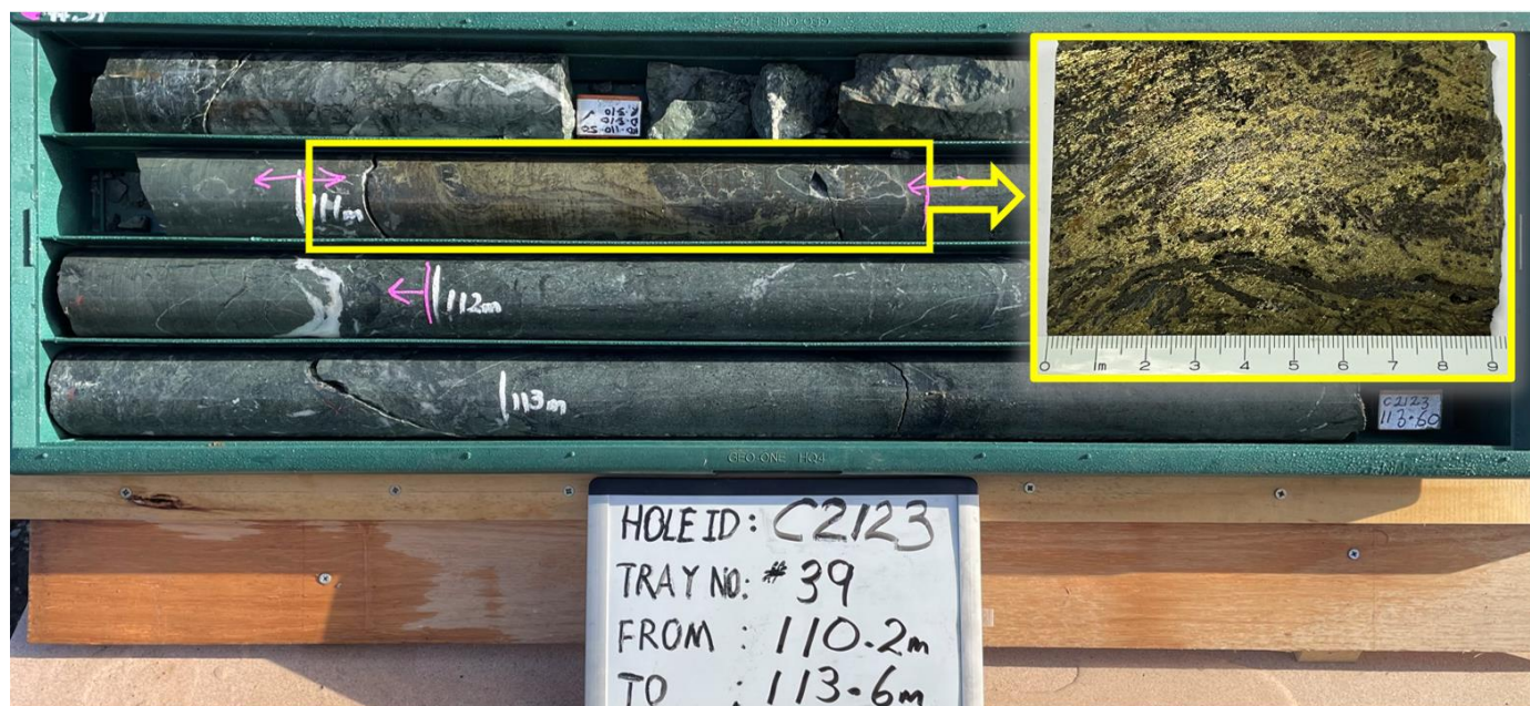
Figure 6. Drill hole C2123 depicting, with the yellow box indicating the semi-massive copper sulphide mineralisation from 111.0m – 111.45m.
