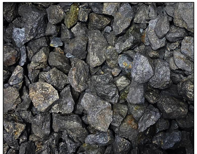
Photo 1. Mined and coarsely crushed Montezuma mineralisation. Representative sample assays of mineralisation only batches averaged 9.02% antimony (Sb), 769 g/t silver (Ag) and 15.47% lead (Pb)
