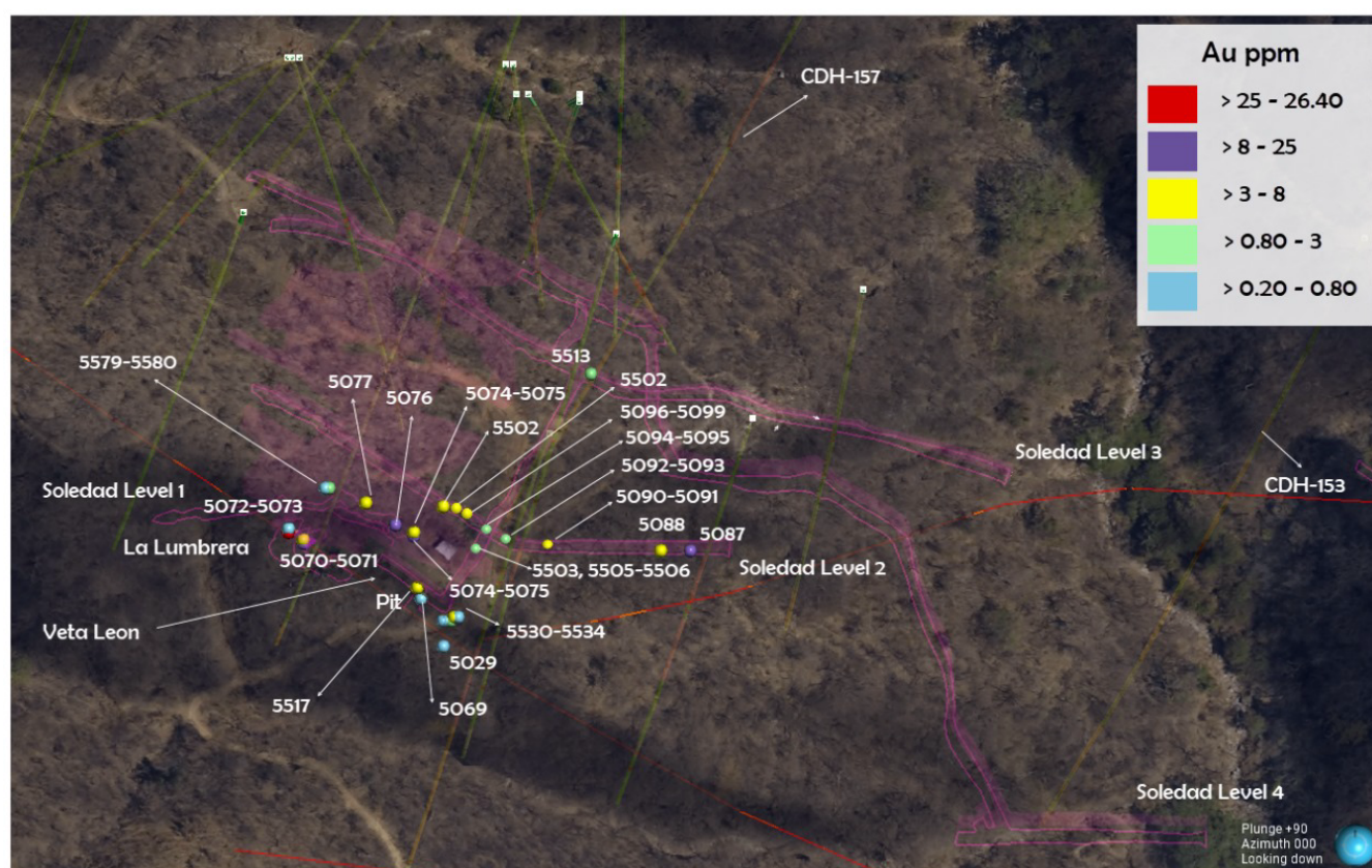
Figure 4 La Soledad workings underground channel sampling (Target 1 area)
