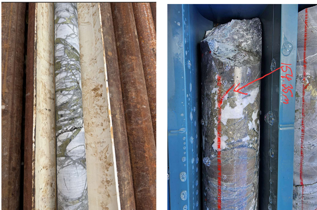
Figure 2. Chalcopyrite/Pyrite infill breccia examples from hole 24
