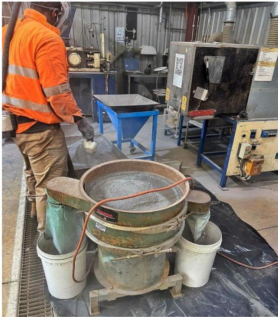
Figure 3: Screening of crushed material
