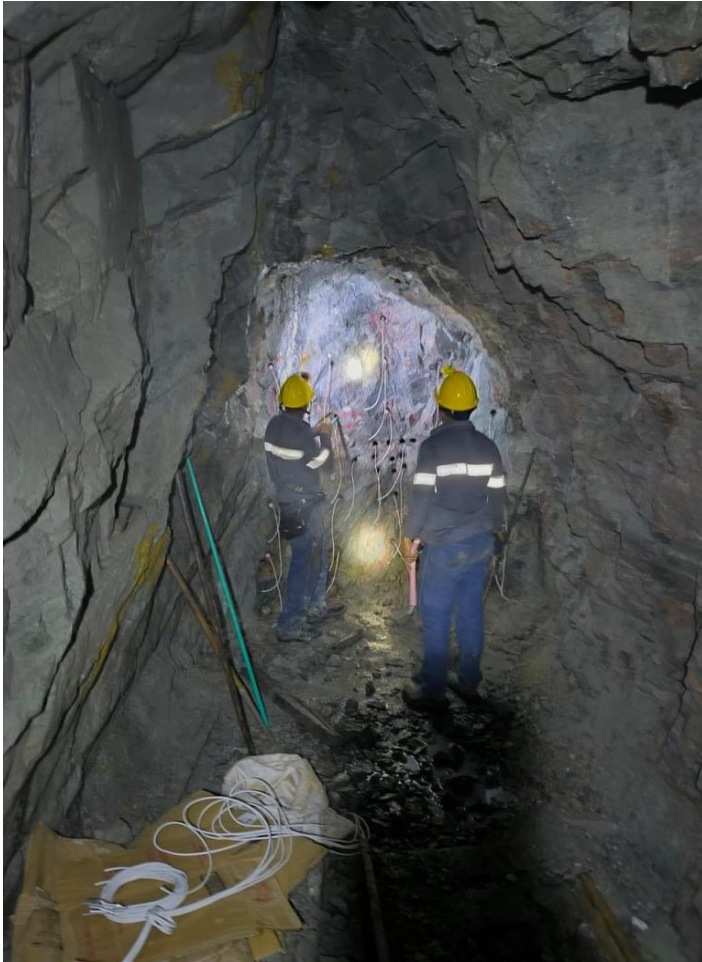
Development Drive Wired for Blasting
