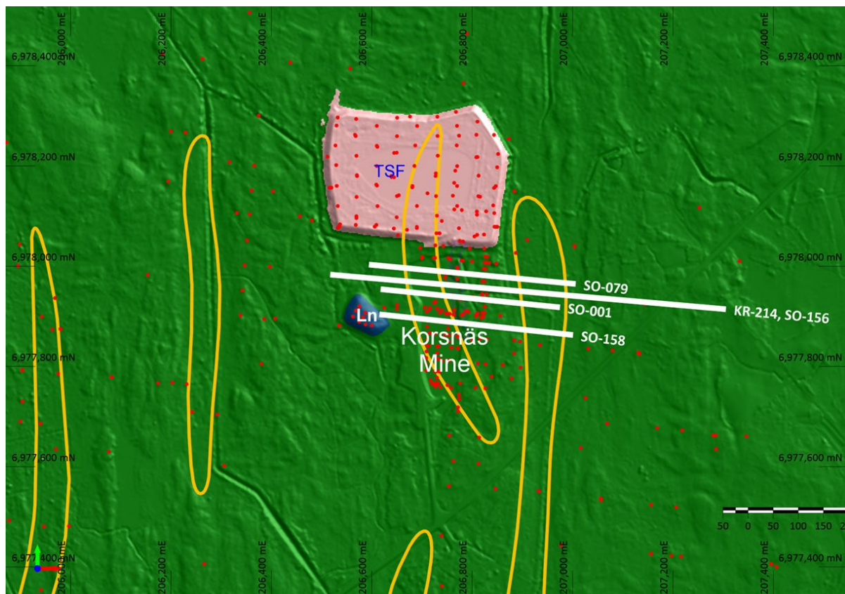
Figure 1. Map showing the locations of drill sections presented in the following figures at Korsnäs. Gravity-low anomalies, which correlate well with near-surface mineralisation, are highlighted by yellow ellipses. The Tailings Storage Facility (TSF), Lanthanide Concentrate Stockpile (Ln), and all drill collars (red dots) are also shown.
