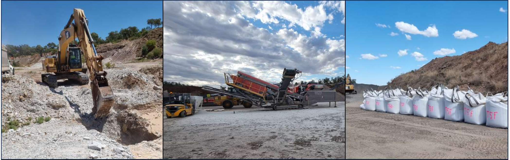
Figure 1: Left – Excavating the bulk sample from trench T7 and loading directly into a waiting truck; Middle – Sample being loaded into the crushing and screening plant in Condobolin, where the sample was crushed to -40mm and screened to separate the -7mm fines; Right – Sample awaiting transport after being loaded into bulk bags for transport to TOMRA Ore Sorting Solutions, Sydney for full-scale ore sorting testwork before downstream concentrating in pilot-scale processing plants at ALS Perth and then ALS Burnie.
