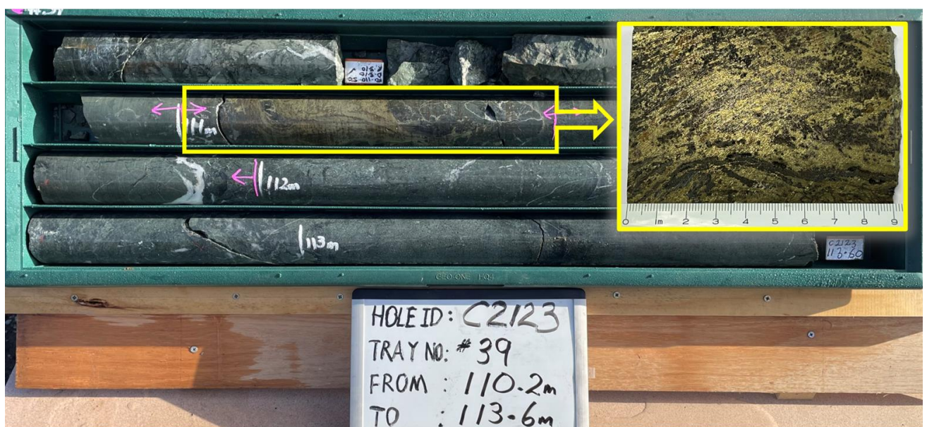
Figure-3. Drill hole C2123 depicting, with the yellow box indicating the semi-massive copper sulphide mineralisation from 111.0m – 111.45m
