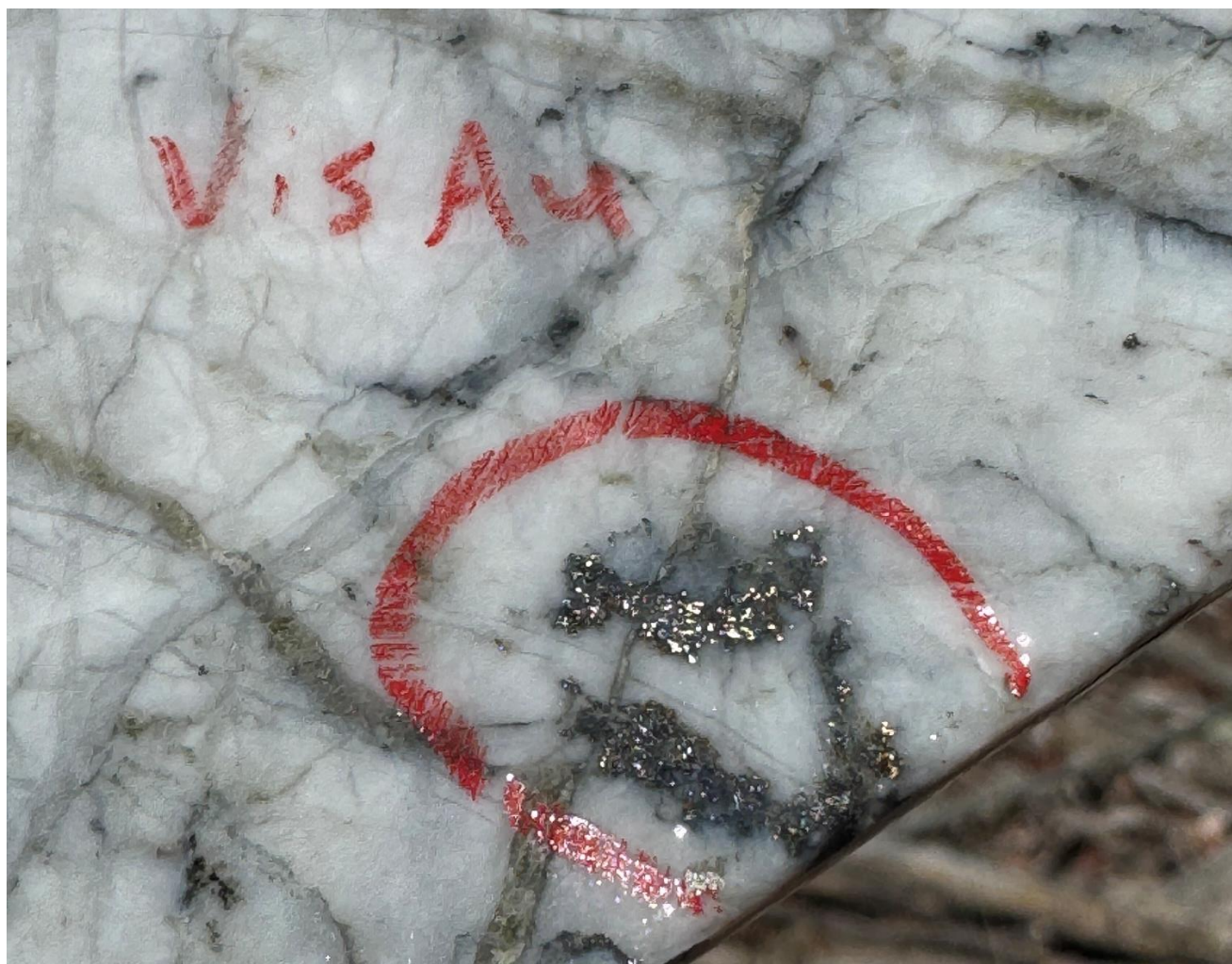
Figure 2. Abundant visible gold 2 grains (lustrous yellow) in an irregular patch of sulphides (grey/black) from a cut section of AMD001 core at 189.0m. Assays are currently pending for this hole.
