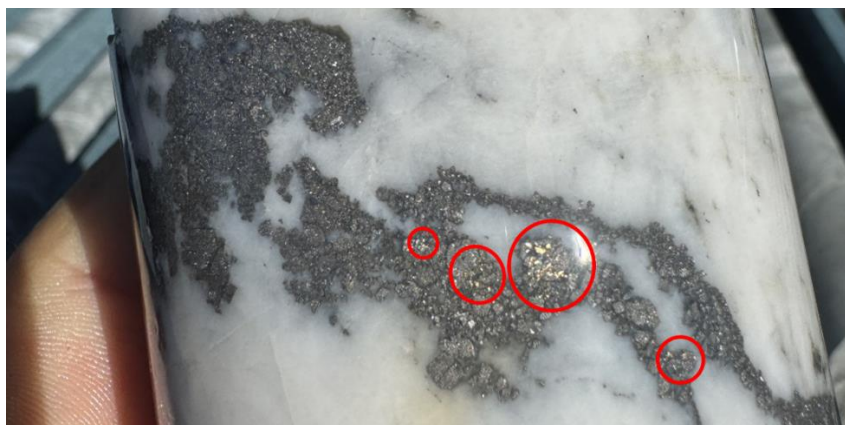
Figure 1. Diamond drill core from AMD003 at 180.0 metres down hole showing abundant grains of visible gold 2 (yellow) hosted within an arsenopyrite vein (grey) in milky quartz. Assays are currently pending for this hole.
