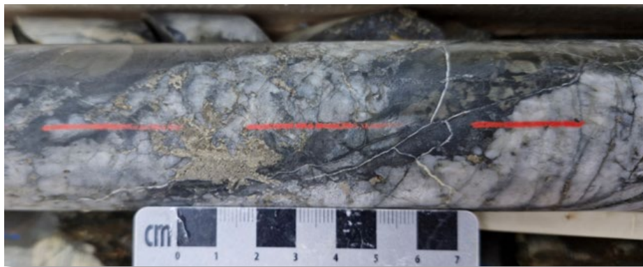
Figure 10. CUTBD03, 145m – Unsampld pyrite(brass-yellow)-pyrrhotite (brown-bronze) in quartz vein iii (see Cautionary Note Page 6).
