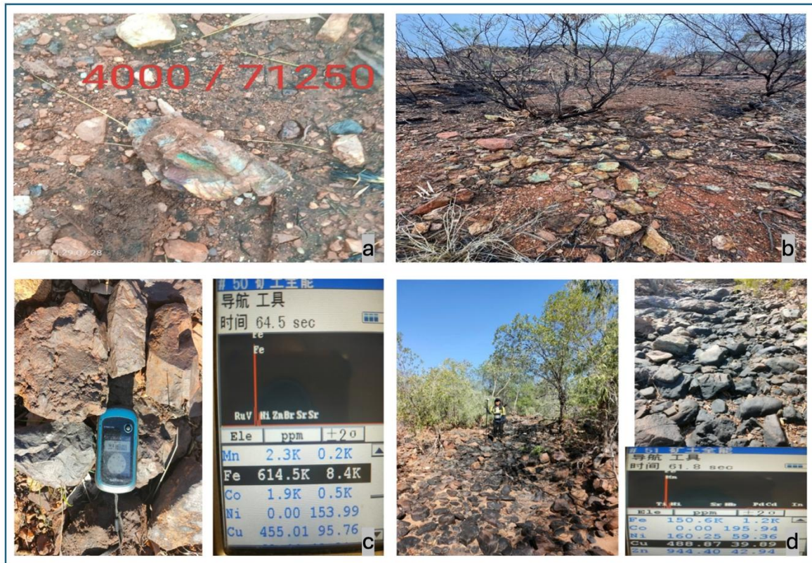
Figure 5: Photos illustrating high grade oxidized copper ore, mainly malachite (a, b), magnetite quartzite (c) and meta-mafic unit). Note that P-XRF analyses reading are indicative only for guiding further test work.
