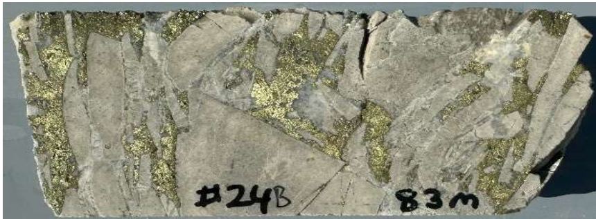
Example of high grade chalcopyrite infill in hornfels breccia. CAE Hole 24, 83m . 2m interval 82m-84m : 3.04% Cu, 0.23 g/t Au, 102.9 g/t Ag, 4.11% S (2m @ 4.0% CuEq).
