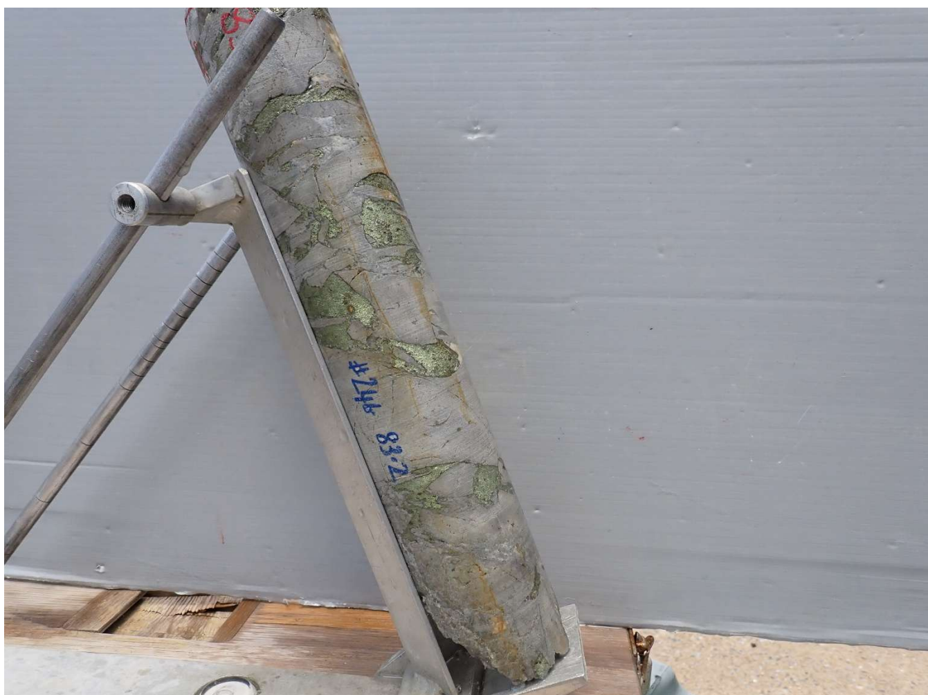
Fig 13. Photo full HQ core Hole CAE 024, selected interval oriented in core oriented frame at 83.2m, hole drilling to west south west , view looking south east , hole at 83m inclined at -68 degrees toward 248 degrees mag: Chalcopryite rich Hydrothermal Infill Breccia. Clasts dominated by yellow grey, sericite altered hornfels, with infill of chalcopyrite (golden) , pyrite (brassy) ,minor calcite (white) ,quartz (glassy).
