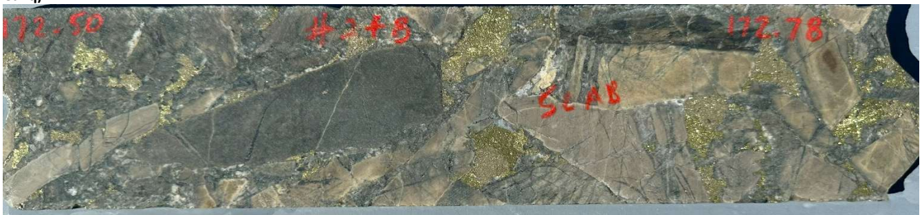
Example of infill polymict hydrothermal breccia, dominated by hornfels clasts, with chalcopyrite (golden), pyrite (brassy), quartz calcite, rock-flour infill. CAE Hole 24, 172.5m. 8m interval 170m-178m : 0.98% Cu, 0.26 g/t Au, 11.2 g/t Ag, 4.25% S. (8m @ 1.23% CuEq).
