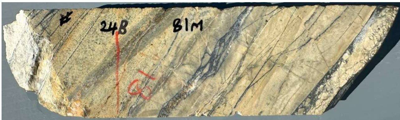
Fig 12. Photo Half HQ Core . Hole 25CAEDD024 selected interval at 81m - sericite altered and heavily veined hornfelsed siltstone with prominent sheeted veins of quartz-ankerite-pyrite-molybdenite -minor chalcopyrite. -1m interval 81m-82m : 666 ppm Mo, 0.11% Cu, 0.02 g/t Au, 1.3 g/t Ag, 0.5% S.
