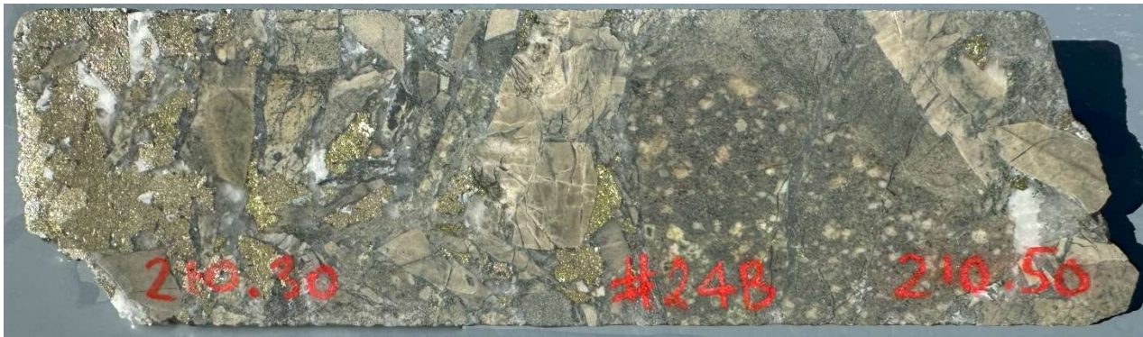
Example of infill polymict hydrothermal breccia , hornfels & porphyry clasts, with chalcopyrite (golden) , pyrite (brassy), quartz calcite, rock-flour infill. CAE Hole 24, 210.5m. 1m interval 210m-211m : 0.60% Cu, 0.20 g/t Au, 7.9 g/t Ag, 7.68% S. (1m @ 0.78% CuEq).
