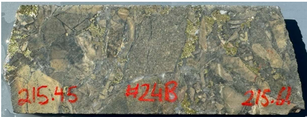
Example of infill polymict hydrothermal breccia, dominated by hornfels clasts, with chalcopyrite (golden), pyrite (brassy), quartz calcite, rock-flour infill. CAE Hole 24, 215.5m.5m interval 212m-217m: 0.35% Cu, 0.07 g/t Au, 3.6 g/t Ag, 2.80% S. (5m @ 0.42% CuEq*).
