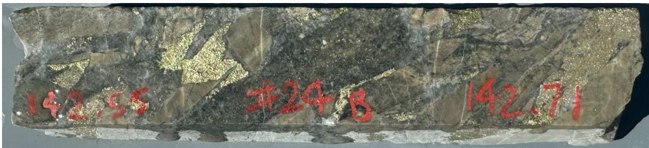
Example of infill polymict hydrothermal breccia, dominated by hornfels clasts, with chalcopyrite (golden), pyrite (brassy), quartz infill, some altered porphyry. CAE Hole 24, 142.5m. 4m interval 141m-145m : 1.42% Cu, 0.49 g/t Au, 12.8 g/t Ag, 4.34% S. (4m @ 1.84% CuEq).
