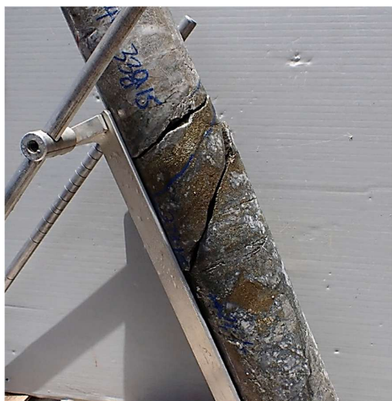
Fig 14. Photo full HQ core Hole CAE 024 ,157.2m, selected interval oriented in core oriented frame, hole drilling to west south west , view looking south east , hole at 157m inclined at -68 degrees toward 251 degrees mag: Infill hydrothermal breccia, with slabby/shingle clasts aligned normal to direction of hole. Slab alignment averages dipping 45 degrees, striking 010 degrees mag , dip direction 100 degrees mag. Clasts dominated by light grey, sericite altered hornfels , with infill of carbonate (white) , quartz (colourless), chlorite infill & altered rock flour (green) , pyrite (brassy) . 1m Interval 157m-158m grades 0.53%Cu, 0.13 g/t Au, 8 g/t Ag, 3.09% S.
