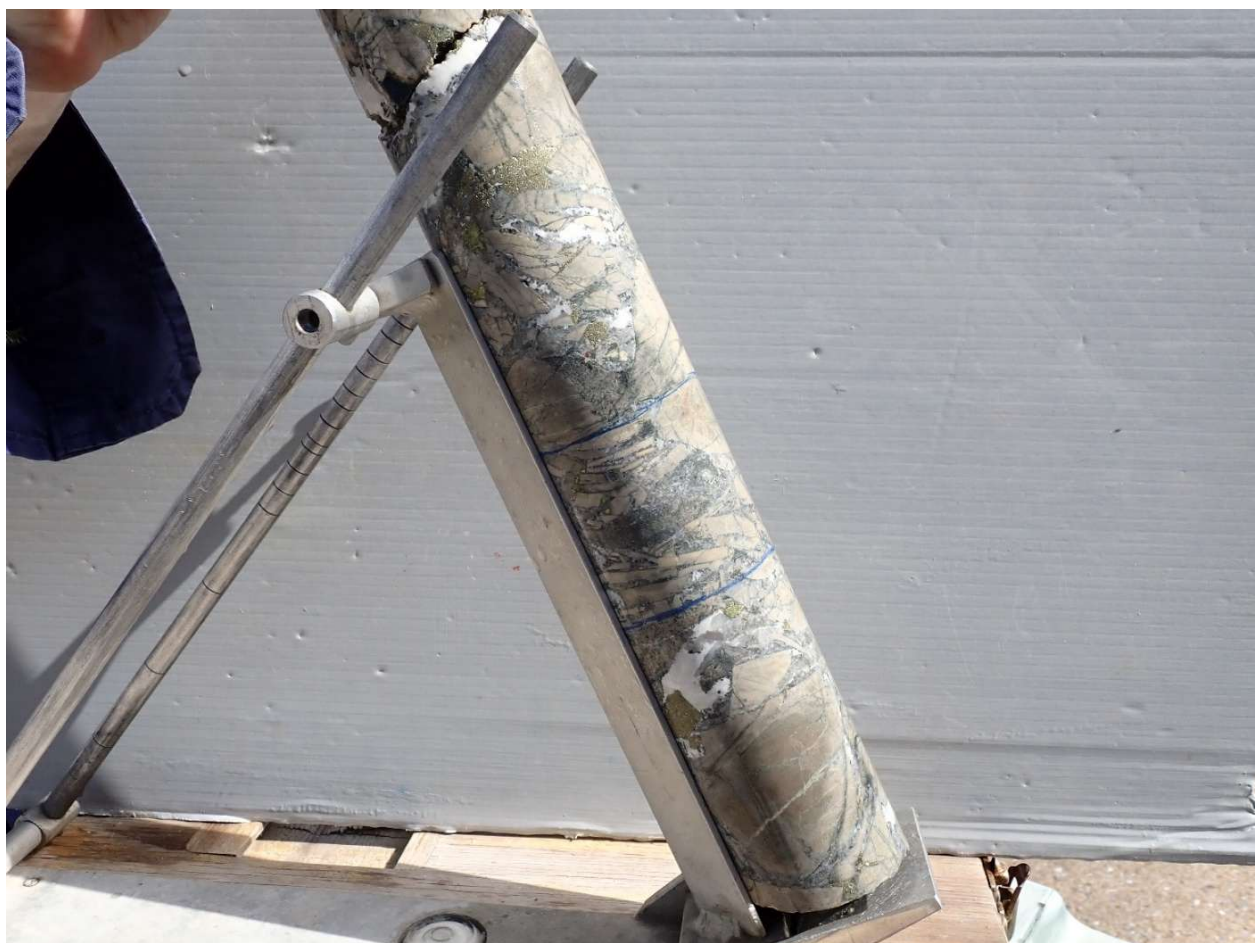
Fig 14. Photo full HQ core Hole CAE 024 ,157.2m, selected interval oriented in core oriented frame, hole drilling to west south west , view looking south east , hole at 157m inclined at -68 degrees toward 251 degrees mag: Infill hydrothermal breccia, with slabby/shingle clasts aligned normal to direction of hole. Slab alignment averages dipping 45 degrees, striking 010 degrees mag , dip direction 100 degrees mag. Clasts dominated by light grey, sericite altered hornfels , with infill of carbonate (white) , quartz (colourless), chlorite infill & altered rock flour (green) , pyrite (brassy) . 1m Interval 157m-158m grades 0.53%Cu, 0.13 g/t Au, 8 g/t Ag, 3.09% S.
