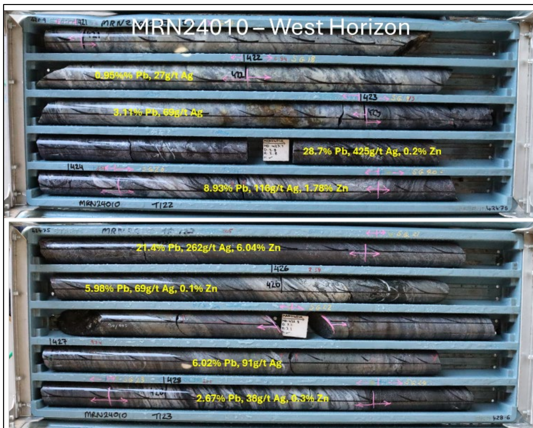
Figure 2. Drill core photos for MRN24010 showing Western Horizon intercepts
