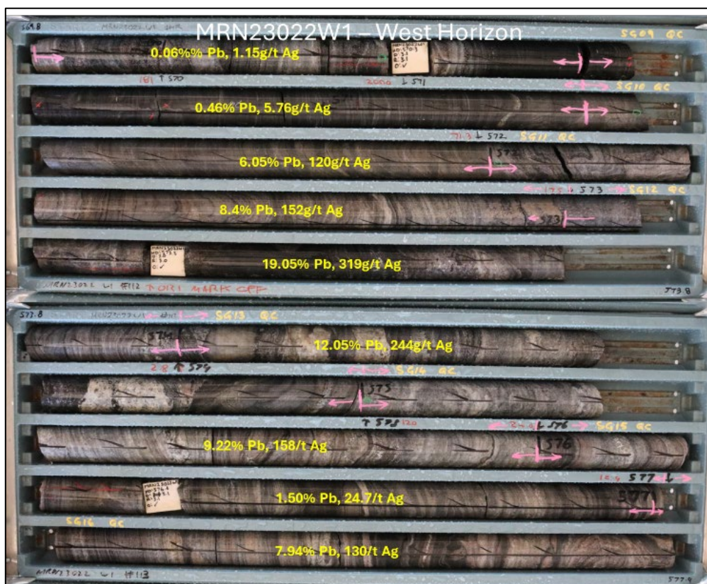
Figure 3. Drill Core photos from MRN23022W1 showing Western Horizon intercepts
