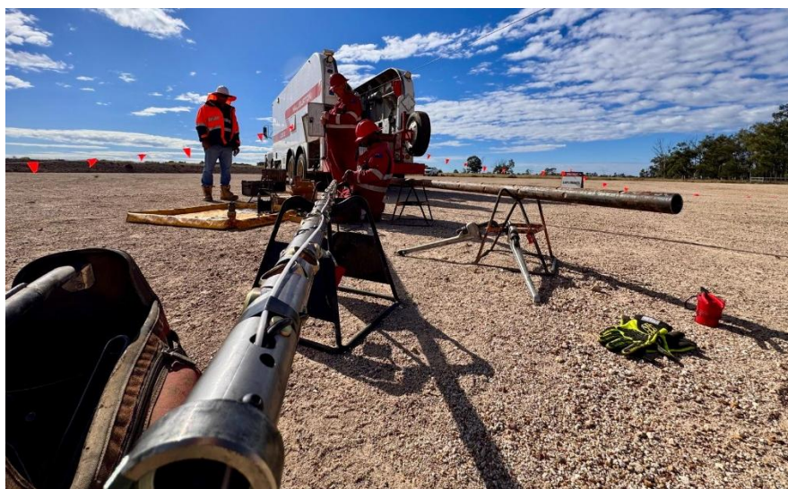
Figure 1 – Loading casing perforation guns in preparation for pumping the first DFIT on Canyon-2
