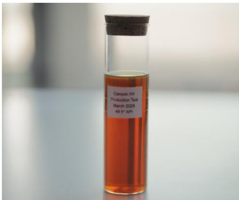
Figure 5 – Crude oil sample from Canyon-1H flow test
