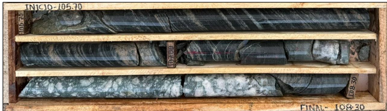
Photo 2. Target mineralized vein #1 (DDH SB-25-01, from 105.7 to 108.3m) intersected under the main Santa Barbara development tunnel (Figures 1 and 2). The vein is comprised of an early quartz and semi-massive pyrite that (almost 50% of the stage 1 vein event) is visible on the vein edges, following right-lateral fault zones. This event is followed by an epithermal reactivation manifested in breccia textures affecting the initial stage and a second generation of quartz and calcite fragments cemented by chlorite and sericite/pyrite alteration halos in the wallrock clasts. Iron poor yellow sphalerite and coarse galena complete the epithermal paragenesis. Assay results are pending.
