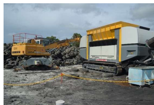
2023: purchase of shredder machine, adding pre-processing capabilities & ability to handle other wastes ~50-60% coal substitution
