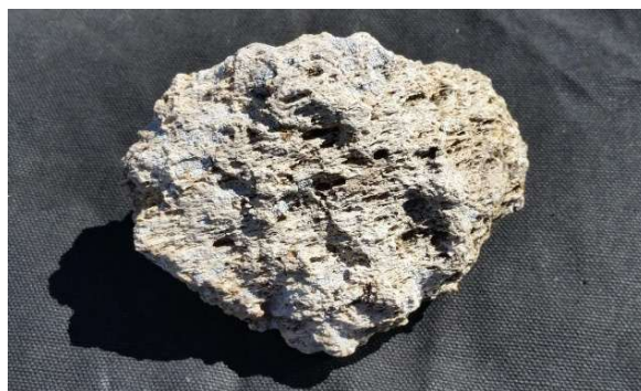
Pozzolans – naturally occurring volcanic materials used in ancient Greek and Roman construction
