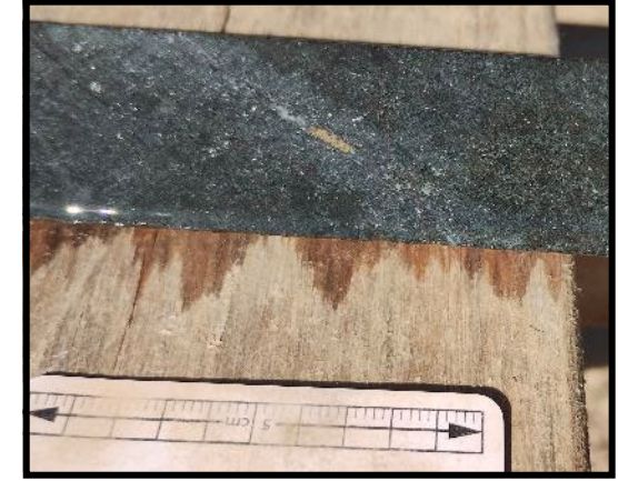
Thin erratic quartz/Cu sulphide veins crosscutting foliation and bedding, BUDD192 @ 130.1m
