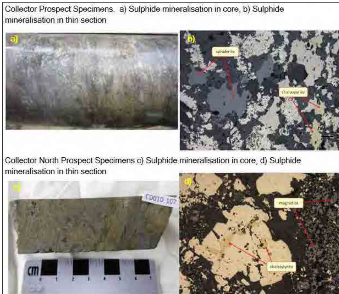
Figure 4-9: Sulphide Mineralisation - Collector and Collector North Prospect
