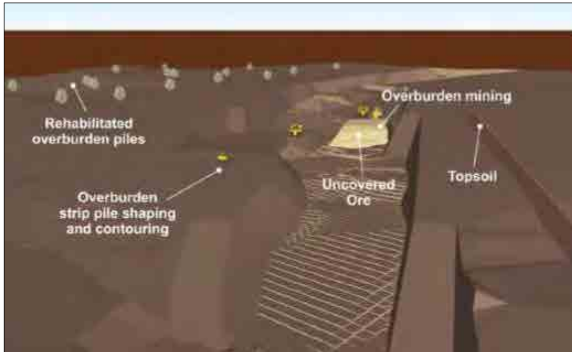
Figure 2-15: Illustration of Strip-Mining Progression (Optima, 2018)
