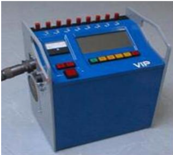
Figure 1: VIP 5000 I.P. transmitter and Receiver
