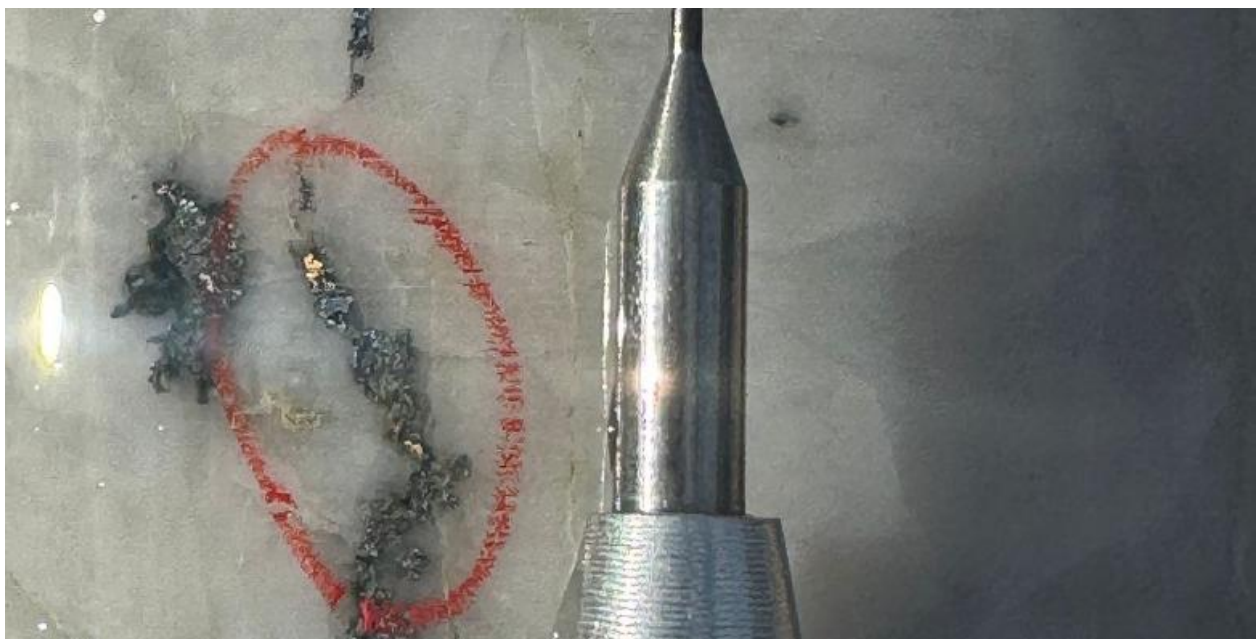
Figure 4. Diamond drill core from AMD009 at 201.6m metres down hole showing grains of visible gold (yellow) to 2mm hosted in an arsenopyrite vein (grey) in milky quartz. This occurs in a zone that graded 3.2m at 44.2g/t Au.
