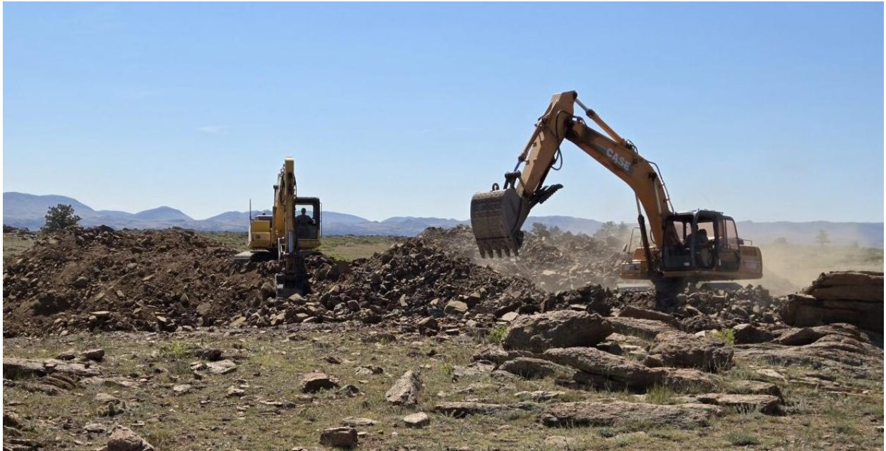
Figure 2 - Excavation of the blasted, weathered material at the CSM Test Mine
