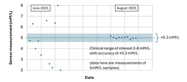
Archer's graphene Biochip has already reached key technical milestones including improvement of variability between gFETs used for sensing(ASX announcement, 25 Feb 2025). The platform has since progressed to human blood testing and early prototype cartridge integration. This graphene-based approach (gFETs) remains central to Archer's vision of delivering a high-performance biosensor product, with clinical trials targeted to commence in 2026.
