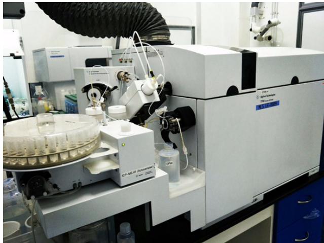
Marchwood's ICP-MS Machine for analysing samples
