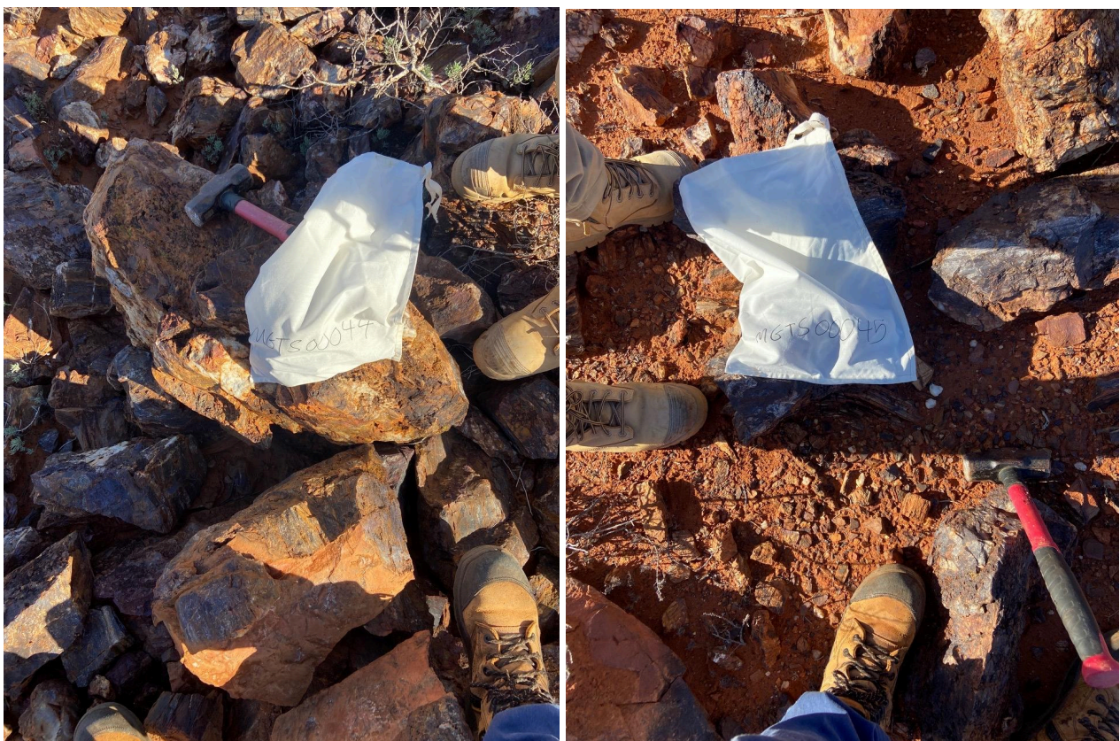
Figure 02: Mineralised samples (MGTS00044 and 45) of fractured, quartz-veined BIF.
