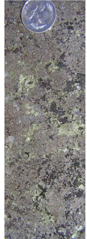
*Discovery drillhole EL 14D09, 166.6m: coarse, massive sulphides including chalcopyrite (yellow), sphalerite (black), pyrrhotite (bronze) and calcite (white to pale grey)*
