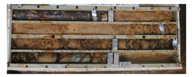
All 6 holes were drilled, as expected, in highly oxidised rock with a stock-work of numerous narrow veinlets of mineralised quartz, iron oxide and manganese oxide.
