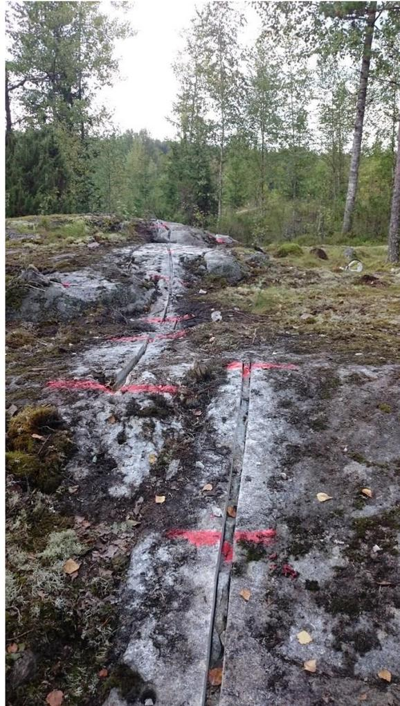
Figure 9: Channel sampling across the main Kietyönmäki lithium pegmatite dyke
