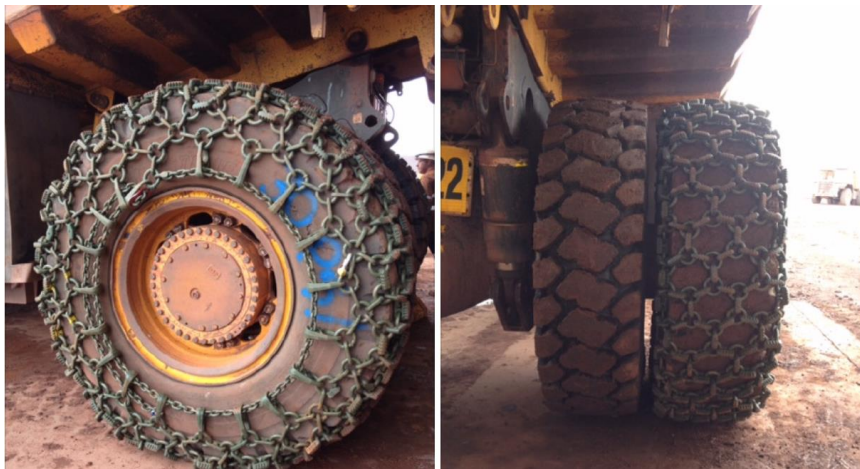
Underground safety improvement plan execution – truck tyre chain trial targeting reduced truck related incidents and improved productivity.
